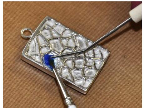
16) Let the enamel dry completely before firing. After it is dry, you can still clean up or refine the edges with a brush.
