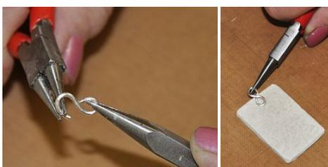
7) Bend 16 gauge fine silver wire into a figure 8 shape of an appropriate size for your clasp.
